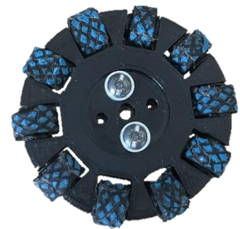
Figure 3: self-made omni wheel
